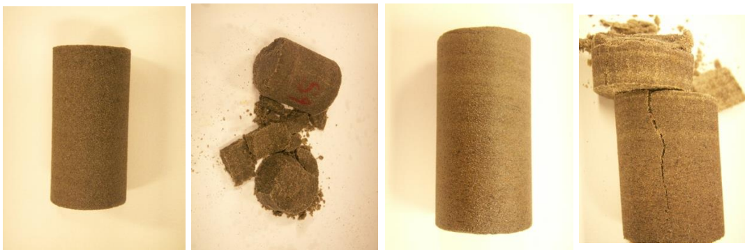
Figure 4. Type of failures induced in the samples under the UCS testing conditions
