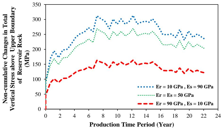
Fig. 2. Differences between Non-cumulative Changes in Total Vertical Stress of Adjacent Area near the Side Boundary of the Reservoir in the Surroundings During 22-year Production.
