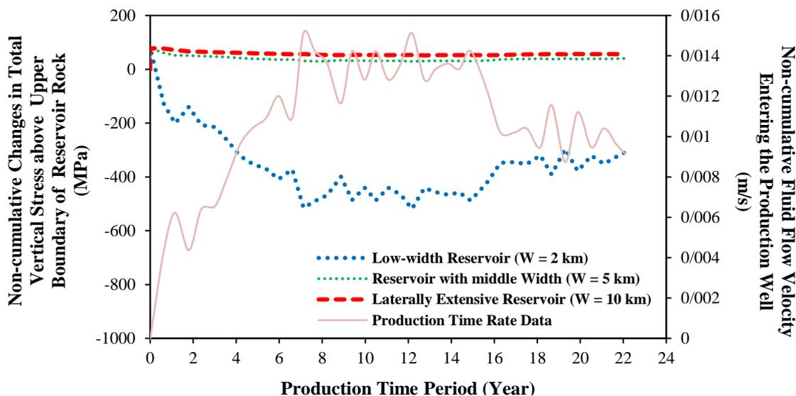
**Fig. 1.** Comparison of the Non-cumulative Changes in Total Vertical Stress Affecting the Upper Boundary of three reservoirs with Different Widths During 22 years of Production.
