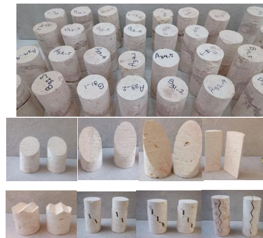
Figure 3. Some of the prepared rock samples in order to conduct confined compressive test
