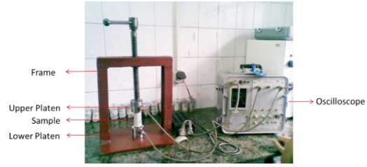
Fig 2. Experimental apparatus for ultrasonic wave velocity measurement.
